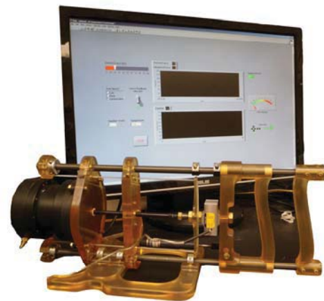
Figure 4. The Variable Resistance Hand Device V3 and its Graphical User Interface.
