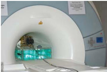
Figure 9. Experimental setup showing the Phantom and Hand Device during imaging
