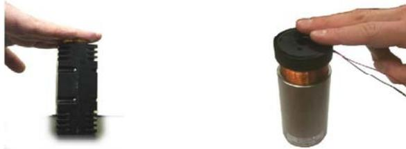
Figure 2: Linear Dielectric Elastomer Actuator (LEFT), Linear Voice Coil Motor (RIGHT)
