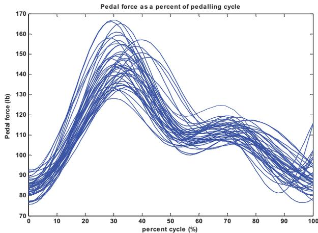
Figure 8: Typical pedal force for one complete pedalling cycle.
