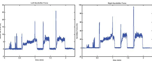
Figure 9: The handlebar forces for the left and right sides while pedalling.
