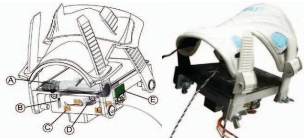
Figure 3: Instrumented pedal module schematic and instrumented pedal module prototype; A: pedal raceway; B: hall-effect sensor; C: pre-load; D: load cell; E: Accelerometer
