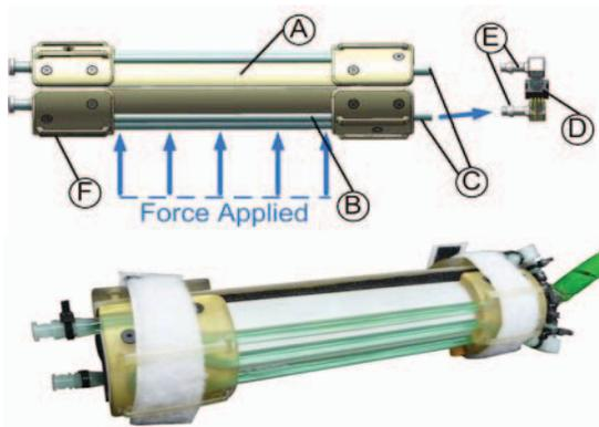
Figure 2: Instrumented handlebar model (top) and prototype (bottom). A: housing; B: sensing area; C: outlet tube sections; D: pressure sensor; E: tubing connections; F: handle caps
