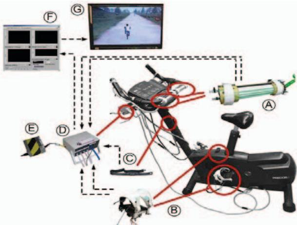
Figure 1: Bicycle system complete overview; A: handlebar module; B: pedal module; C: heart rate monitor; D: signal box; E: power box; F: practitioner interface; G: virtual environment
